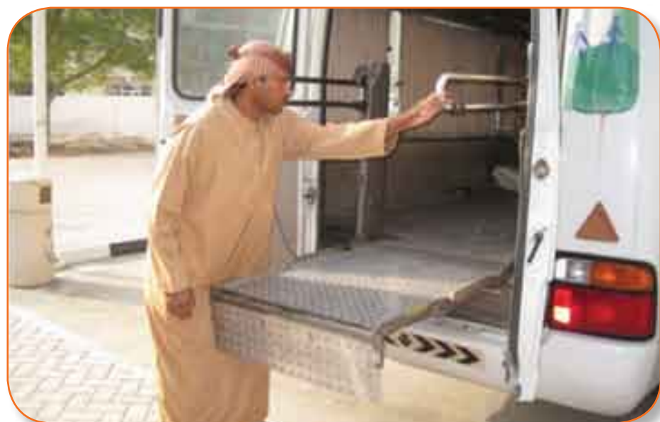
The lift/ramp are designed with safety edges and slip resistance surface.
